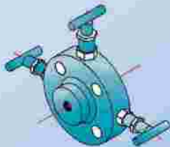
MONOFLANGE-DOUBLE BLOCK & BLEED
